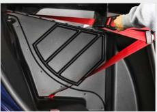
3-Point Pro-straint Harness prevents need to reach across the detainee when buckling.
